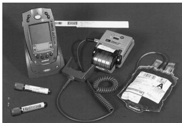
Fig. 1. Safe Track equipment, including wristband with PDF barcode, label printer, and hand-held computer.
